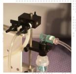
The anesthetic gas flow can be diverted toward 2 independent devices (i.e., an induction chamber and a breathing mask).
