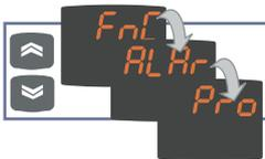
After pressing the “fnc” key, the UP and DOWN keys can be used to scroll through the folders in the menu
