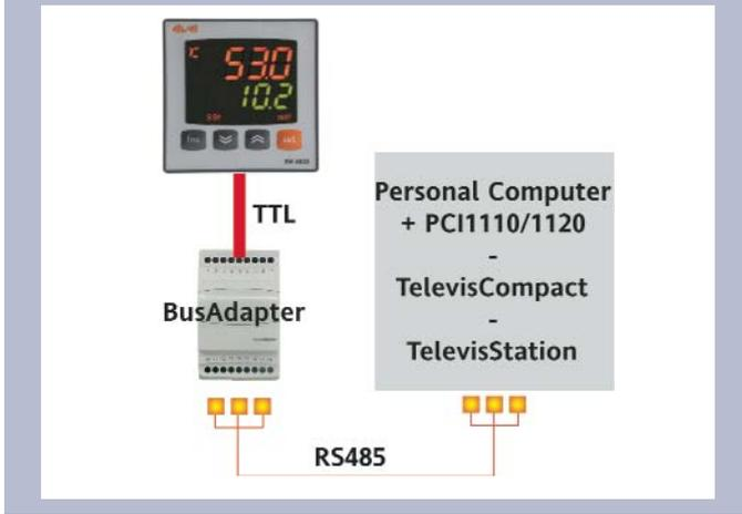
The device can be connected to Televis remote control systems through a TTL serial port (use TTL- RS interface module 485 BUS ADAPTER 130 or 150) or, in models where provided for (EW4822), by means of direct RS485 connection. To configure the device for this purpose, open the folder identified by the "Add" label and use parameters "dEA" and "FAA".
