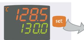
① When the initial display is present, press and release the Set key.
