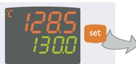
**1** When the initial display is present, press and release the Set key.
