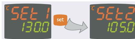
**2** The **PV display** shows label **SET1**, and the **SV display** shows the current Setpoint value. Press the Set key again to display the Setpoint 2 in the same way.
