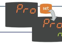
When a label is selected, the Set key can be pressed to access the corresponding folder.
