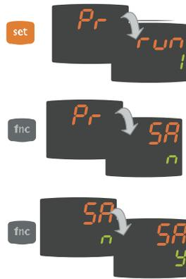
Press the Set key on the desired subfolder to access the parameters. To scroll through the parameters, use the Set key, and to change a value, use the UP and DOWN keys.
