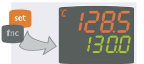
**4** When the Set or "fnc" key is pressed, or the timeout has elapsed (15 sec), the new value appears and the initial display returns
