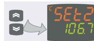
**3** The UP and DOWN keys can be used to change the Setpoint value shown on the **SV display**.
