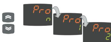
When the desired program has been set, it can be activated by selecting the special **StEP** function in the Functions folder.
