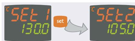
② The **PV display** shows label **SET1**, and the **SV display** shows the current Setpoint value. Press the Set key again to display the Setpoint 2 in the same way.
