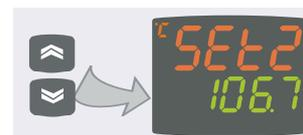
③ The UP and DOWN keys can be used to change the Setpoint value shown on the **SV display**.
