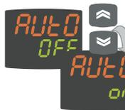
To change the status of a function, use the UP and DOWN keys.
