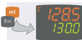
④ When the Set or "fnc" key is pressed, or the timeout has elapsed (15 sec), the new value appears and the initial display returns
