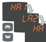
If there are alarms present, the UP and DOWN keys can be used to scroll through and display them
