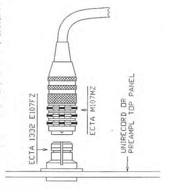
snaps easily out by a combined pull on it and push on the connector body. Use forefinger and thumb of both hands.
