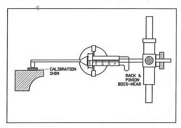
Reposition the stylus on the base line via the balance or the zero suppression knob (see 7050 or 70/9082 instruction manuals).
