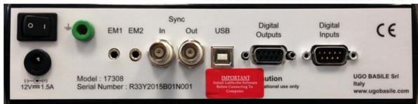
Each channel of the 17308 is equipped with dual, low voltage, independently programmable 16-bit +/- 15V stimulators.
