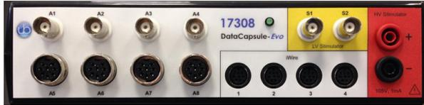
The Maximum sampling speed is 100k samples per second aggregate.
