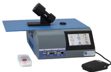
Tail Flick Unit - Thermal stimulation, D'Amour & Smith method
