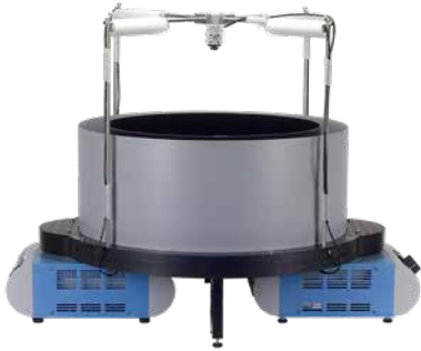
TGR - Thermal Gradient Ring (Zimmermann's method)
