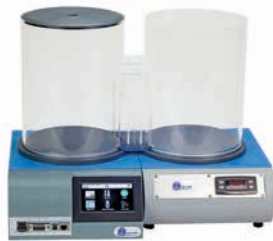
The original Plantar Test for thermal stimulation (Hargreaves Apparatus)
