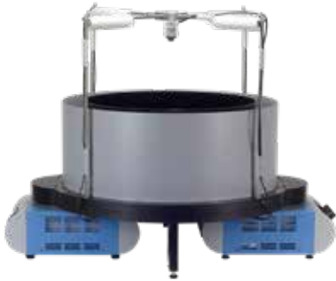
TGR - Thermal Gradient Ring (Zimmermann's method)
