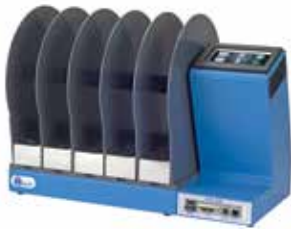
The 1st, original Mouse RotaRod for motory coordination studies
