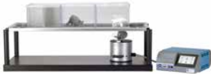
Dynamic Plantar Aesthesiometer (DPA) for mechanical stimulation
