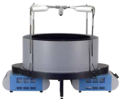
TGR - Thermal Gradient Ring (Zimmermann's method)
