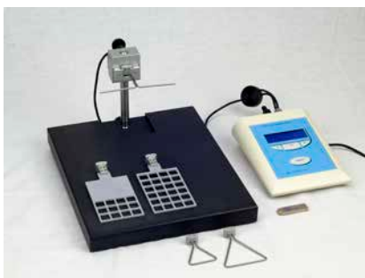
GSM Grip-Strength Meter for mice and rats
