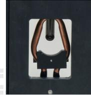
The **mechanical stimulator** relies on thin wires attached to a mounting plate. The system comes with several plates, each with a different number of wires in order to apply different force levels to the animal vibrissal pad.
