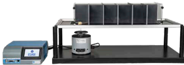
Dynamic Plantar Aesthesiometer (DPA) for mechanical stimulation
