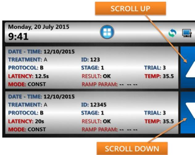
The test results appear under the red headings:
