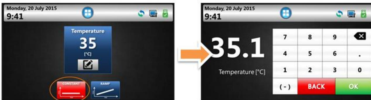
Depress the icon
