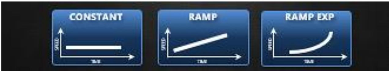
**CONSTANT:** when this mode is selected, the plate maintains the preset temperature
