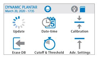
The UPDATE menu requires to insert the USB pen drive and it is necessary to update the device firmware.
