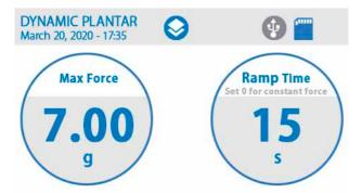
From the "Start" menu, select the operating mode (manual or automatic paw withdrawal scoring) and press the start button to start the force (alternatively, press the button on the touch stimulator unit).
