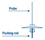
Now remove the probe and put the 5g, 50g and 100g weights on the needle (pushing rod) according to the instructions prompted on the screen. The wizard will take you step by step until the process is completed (see figure below).
