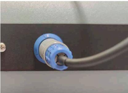
When the sensing cylinder is not connect as show, a yellow alert triagle will appear on the touch screen indicating the missing connection.
