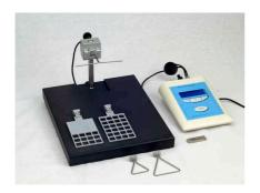
GSM Grip-Strength Meter for mice and rats
