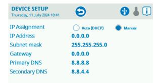
Exit the Network page pressing the rounder arrow on top of the screen.
