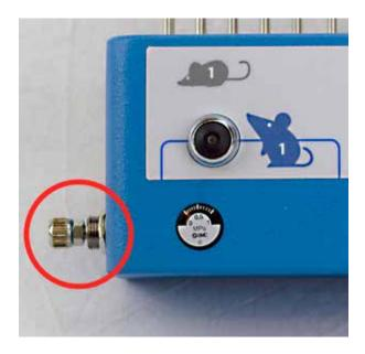
Turning the handle you can adjust the pressur of the AirPuff reading the value on the manometer; depending of the pressure of your air delivery system you will have different possible values.
