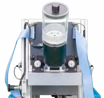
Pellet dispenser (for each chamber)
