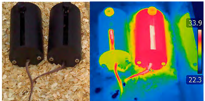
Visible and thermographic vision of experiment with heated and non-heated Romanovsky Holder
