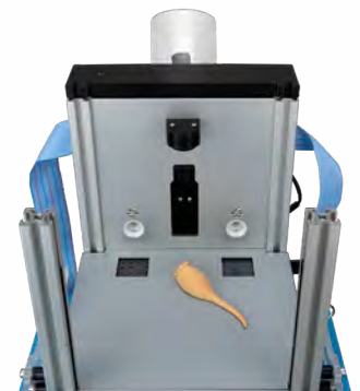
Operant wall and floor
