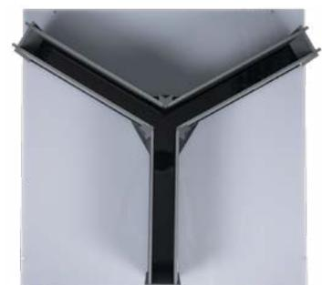
Y-maze with IR transparent walls and floor on LUX IR Illuminator
