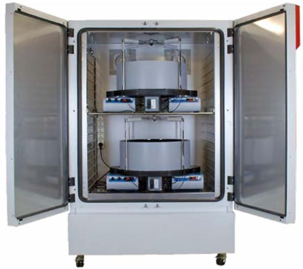
Thermal Conditioned Cabinet for Thermal Gradient Ring
