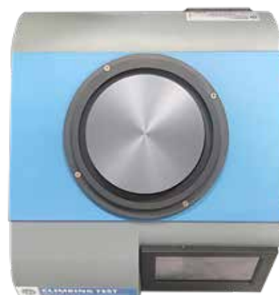
Load cell floor
