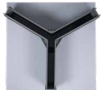
Y-maze with IR transparent walls and floor on LUX IR Illuminator
