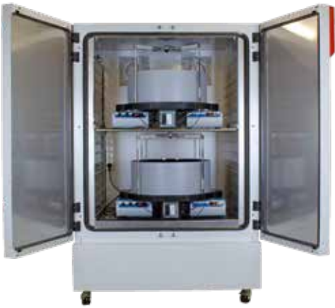
Thermal Conditioned Cabinet for Thermal Gradient Ring
