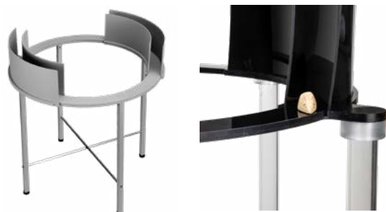
Elevated Zero Maze is available with opaque walls and black IR transparent walls
