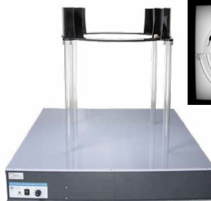
IR Elevated Zero maze and LUX IR Illuminator, with infrared view from the video-tracking software. Notice the exceptional contrast.
