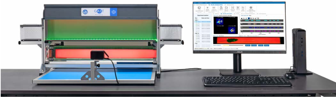
Complete GA.I.T. setup including the GA.I.T. hardware with corridor, 45° mirror, frontal high-speed camera and lateral cages, plus a preconfigured PC with monitor, keyboard and mouse.
