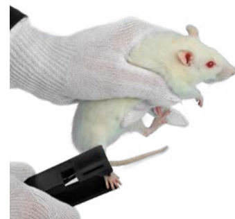
Pressure Applicator (Pincher) option for the PAM used on paw
