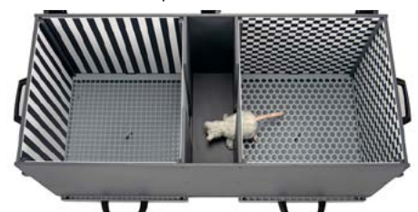
3-compartment CPP, with central neutral area
