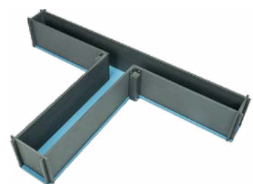
T-Maze with mat plastic walls and opaque metal floor
