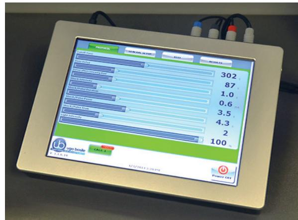
The Unit, incorporating a 12" touch-screen, manages the Passive Avoidance Test via the **40550-010** Software. Up to 4 cages can be connected to the same Controller. If more than one cage is connected, an expansion box **40500-005** is required for each additional cage.
