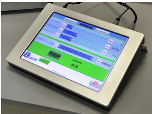
The Unit, incorporating a 12" touch-screen, manages the Passive Avoidance Test via the **40570-010** Software. Up to 4 cages can be connected to the same Controller.
