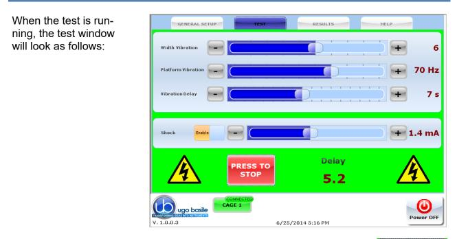
When the animal steps down from the platform, the operator stops the test, and the latency timer by depressing either the "**PRESS TO STOP**" button on the touch-screen, or the pedal switch.
