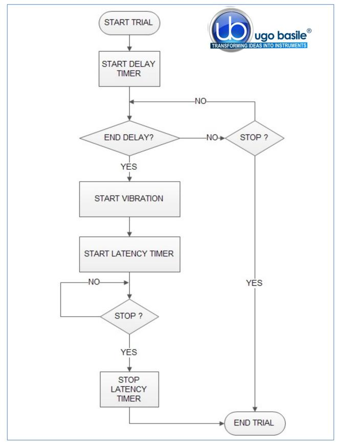
See the following flow-chart, describing the P.A. test (step-down).
