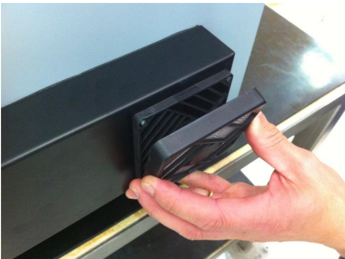
3. Fit in the frame on its housing
