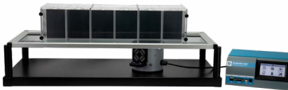
37570 - Plantar Test for thermal stimulation - (Hargreaves Apparatus)
